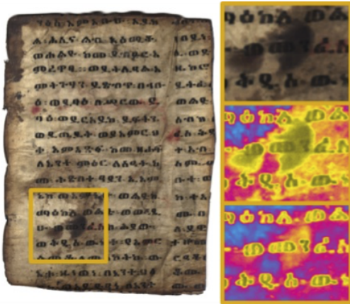
Historical document with heavy soiling, HSI enables the original writing to be made visible (excerpts at 542 nm and 813 nm)
